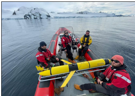
▲ Ocean glider ready to be deployed for a month
