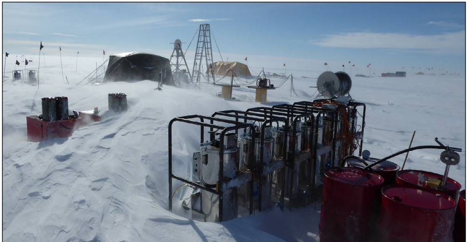
▲ Hot water drilling on Thwaites Eastern Ice Shelf in 2019
