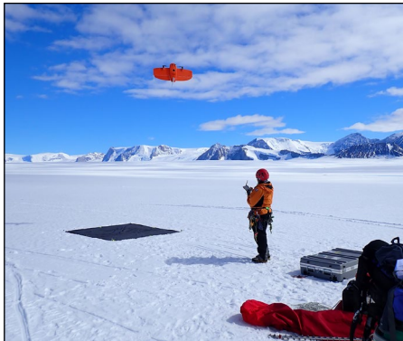
▲ An uncrewed aerial vehicle over Flask Glacier used to photograph the surface and create maps of ice elevation and ice flow
