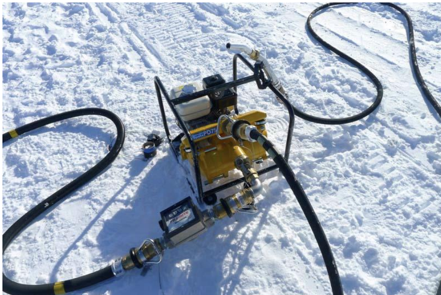
Figure 21. A Spate PD75 pump used for transferring fuel. Source: BAS Traverse Operations Manual.
