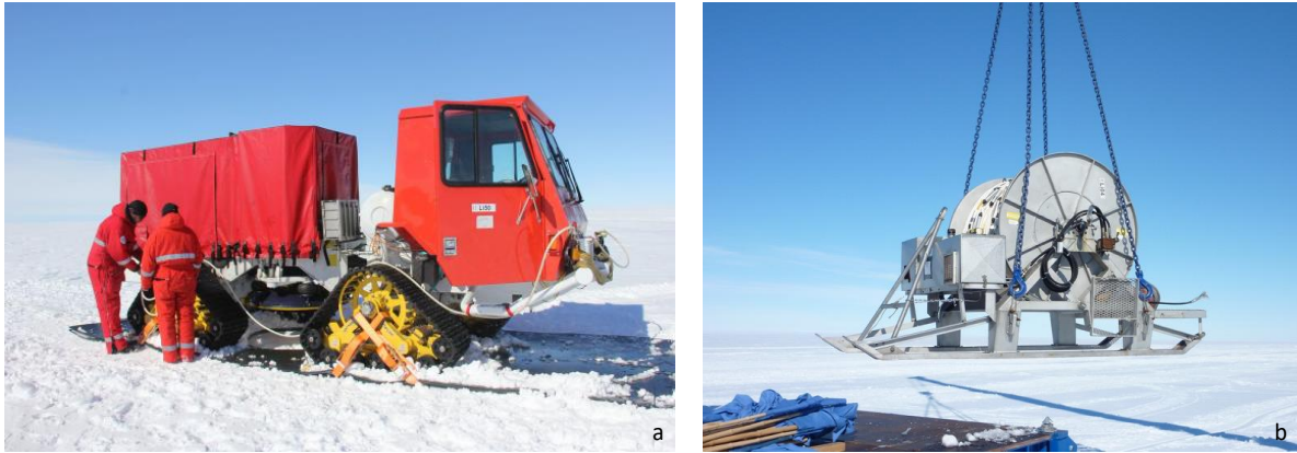
Figure 13. Example of a vibroiseis truck (a) and associated coiled streamer array (b) to be used in a future science traverse. Source: Alfred Wegener Institute
