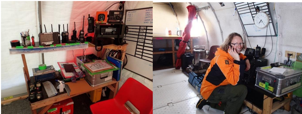
Sky Blu comms station for passing weather observations, talking to Rothera and speaking to inbound aircraft.
