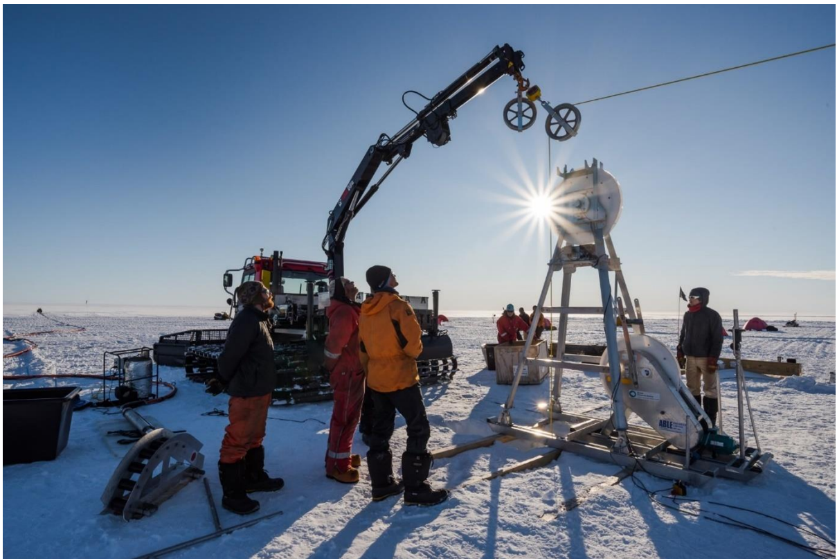
Hot water drilling rig on the joint UK/German FISS project on the Ronne Filchner Ice shelf. Photo: Nick Gillett
