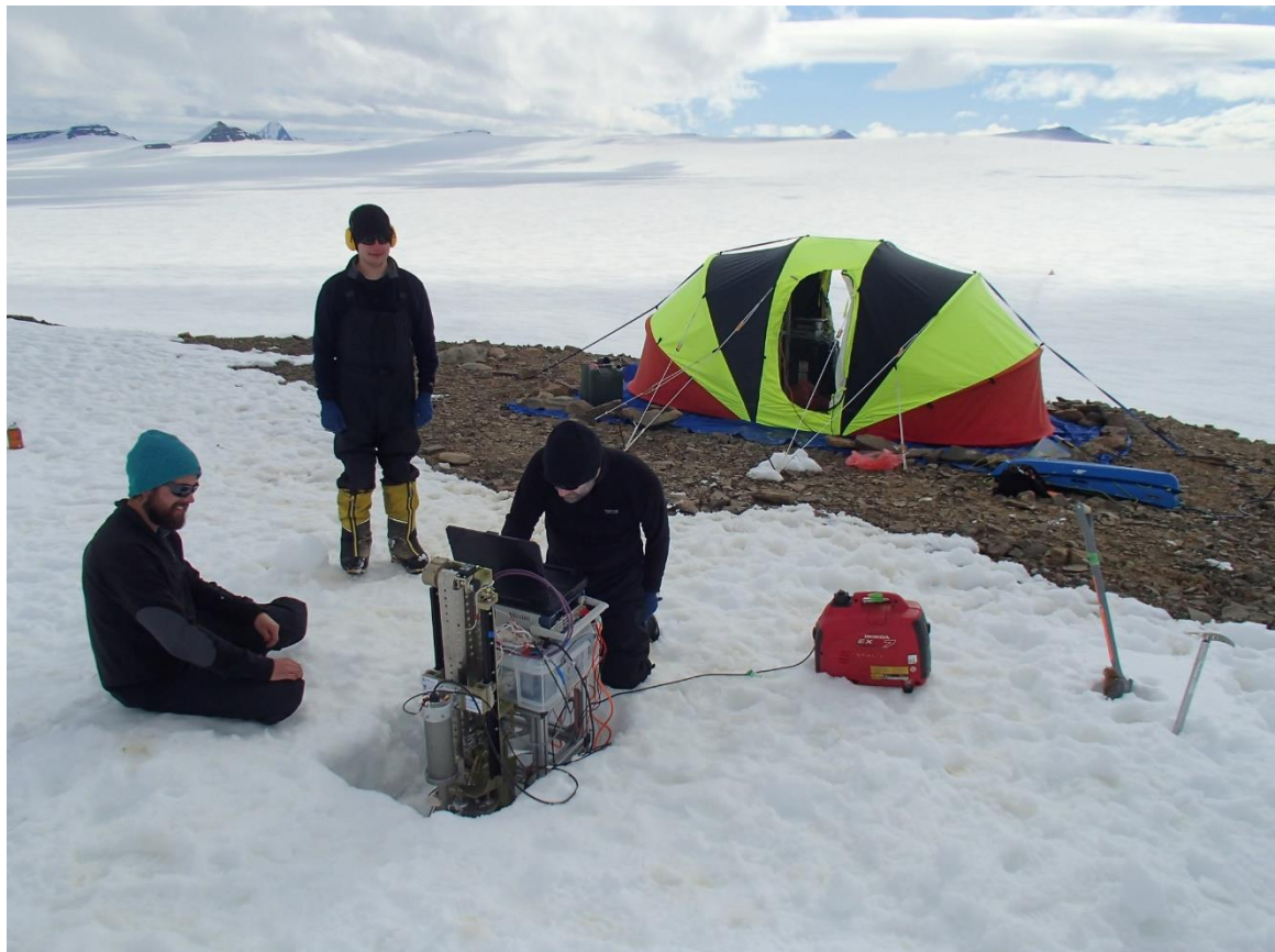
ESA Scientists working with a Mars drill prototype on Coal Nunatak. Photo: Tom Sylvester
