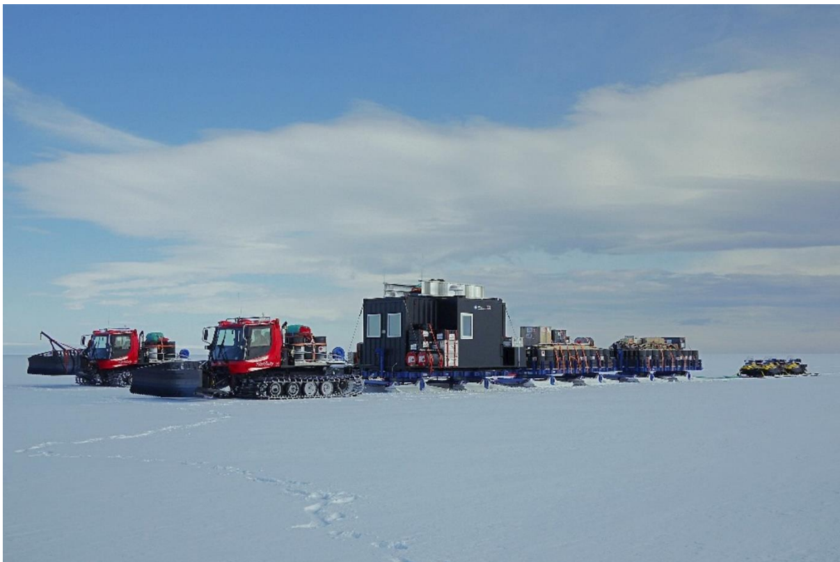
Pisten-Bully towing the living caboose, two sleds of fuel and science equipment and a fleet of skidoos.
