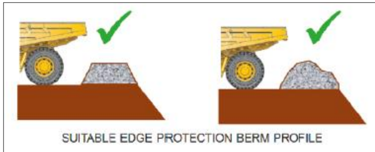
Figure 32 - Example edge protection for tipping operations
