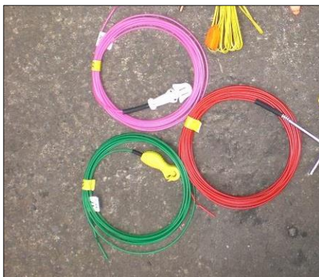
Figure 19 - Examples of non-electric detonators
