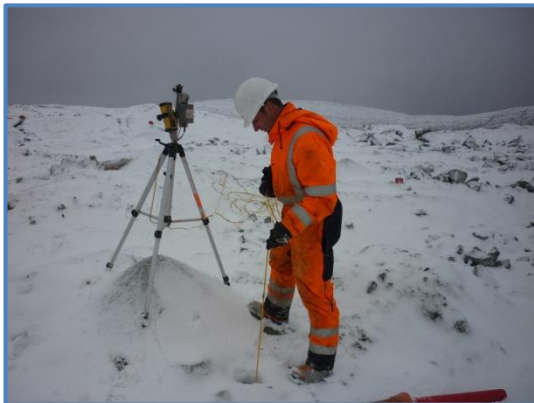
Figure 23 – Surveyor using electronic probe to survey holes
