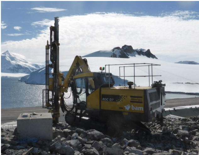
Figure 8 – Atlas Copco D7 tracked drill rig at Rothera.
