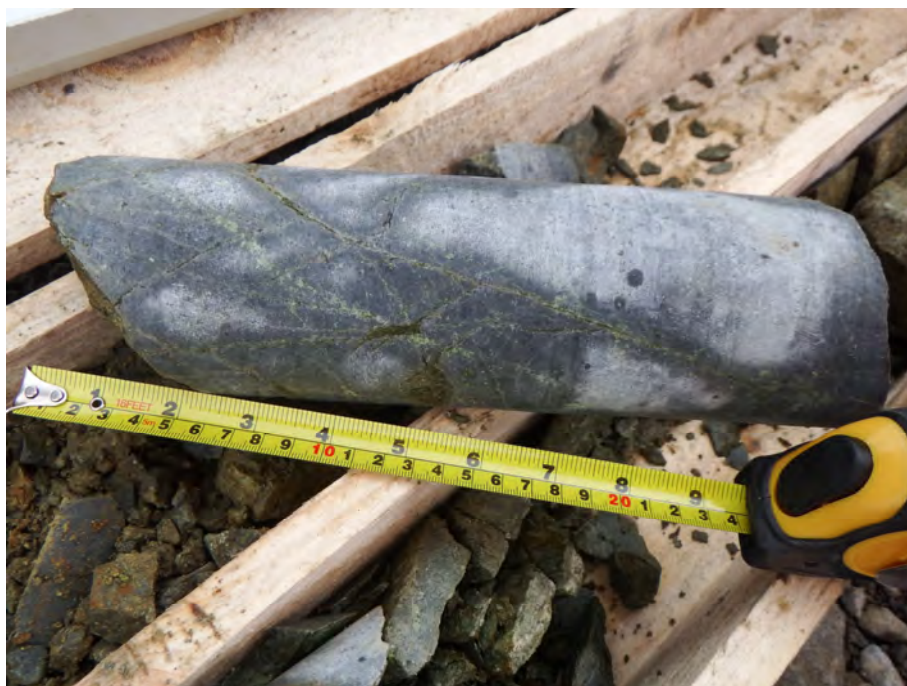
Photo 4 – BHR01 2.65 to 2.95m. Incipient fractures.
