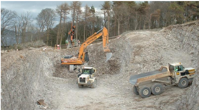
Figure 29 - Example of loading at the face
