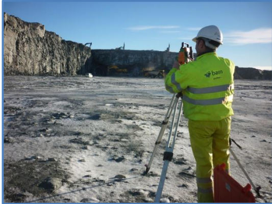
Figure 24 – Undertaking a laser profiling survey of the face
