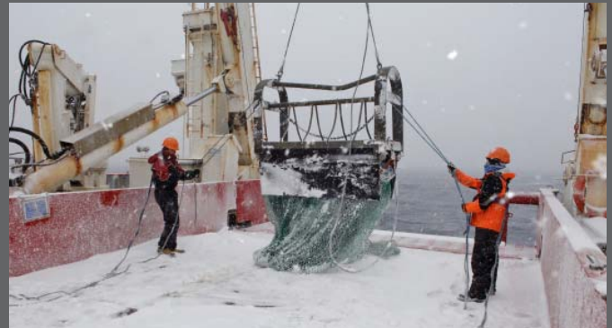
Winch systems have the power to recover heavy instruments and moorings
