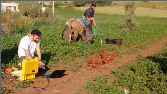
*Working with ground-penetrating radar in Morocco to record groundwater levels*
