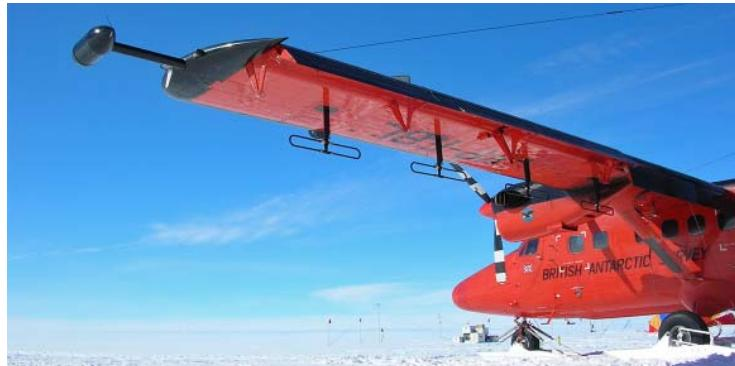
Magnetometer pod and radar antennae on a BAS Twin Otter aircraft
