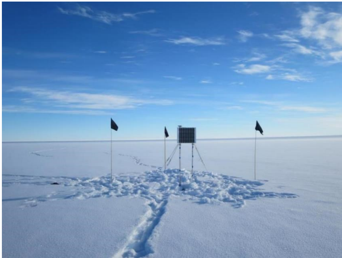
A finished site, each marked with at least two flagged bamboos. The solar panel is mounted on 2 m glacio poles. The zarges box containing the GPS unit, solar regulator and batteries is buried directly behind the solar panel.
