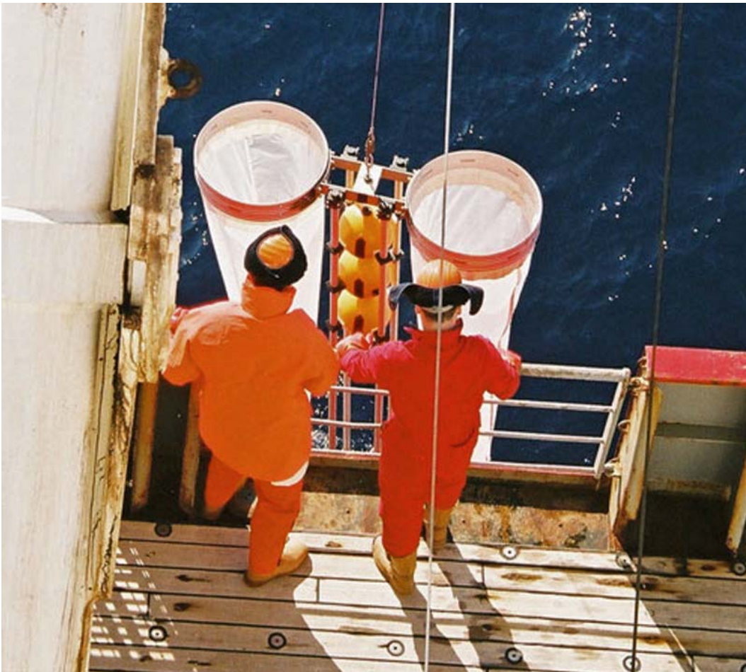
Image: Lowering bongo nets over the side of RRS James Clark Ross .
