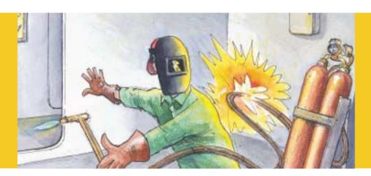
Leave oxy-acetylene equipment alone unless you have been trained to use it correctly. When using oxy-acetylene or other welding equipment, make sure someone knows where you are. Have a fire-watcher, ie an assistant, to stand by with a fire extinguisher to watch for sparks, smouldering or
