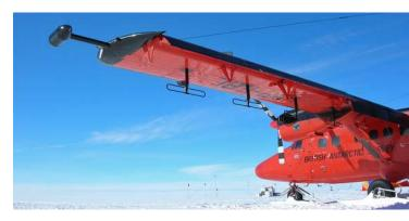
Magnetometer pod and radar antennae on a BAS Twin Otter aircraft
