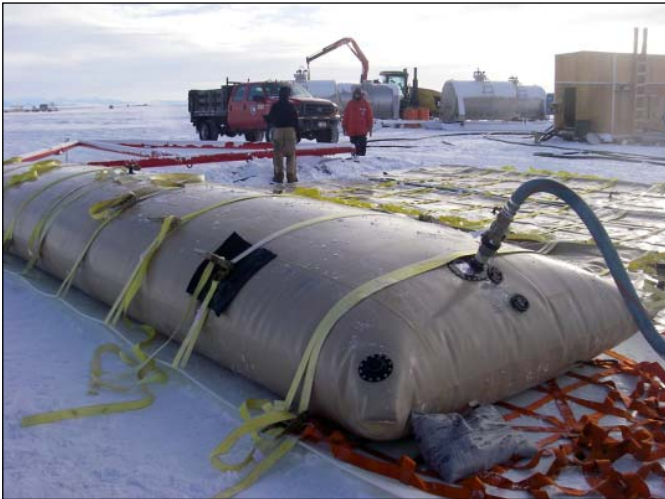
Figure 21. shows an image of the proposed flexible bulk fuel container on a skid base.
