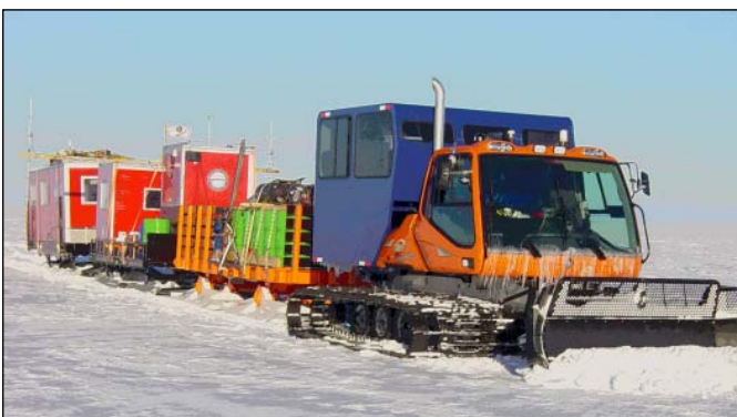
Figure 23. The tractor and sledge used to transport equipment and fuel to the drill site.
